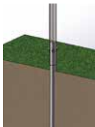
2. Put the post into the ground screw.
